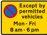
Repeater sign within a loading area
