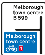
Non-primary route direction sign, in advance of a junction, indicating a route for cyclists
